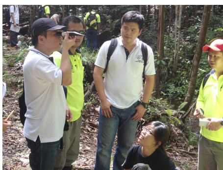
Photo: Students using a refractometer to determine the salinity of the water sampling collected at nearby stream
