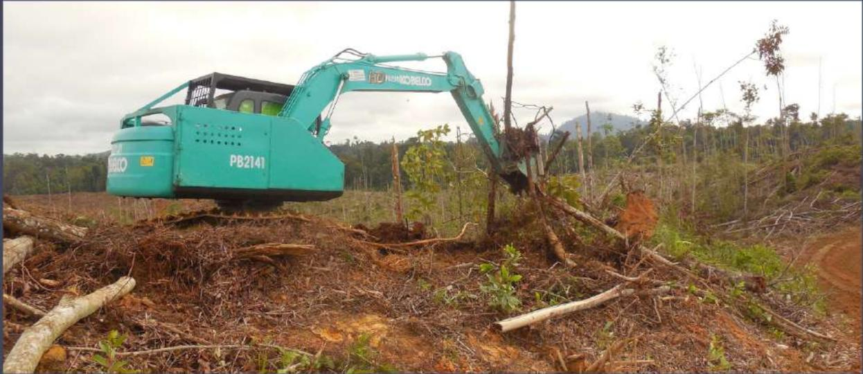
*Skills set: Mechanical Site Preparation – Excavator (Forest Plantation), Activity: Spreading and Crushing at the Plantation Site*
